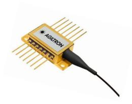
The DFBD series fiber-coupled laser diodes are designed with a GaAs quantum well structure integrated with a grating configuration. These diodes feature a built-in photodiode for precise monitoring and feedback control of the laser's output power. Housed in standard TO packages, these diodes are pigtailed to a 1-meter long single-mode fiber terminated with an FC/APC connector. Each unit undergoes rigorous testing prior to shipment to ensure reliability.
